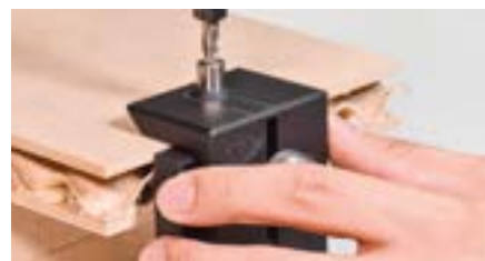
Bedieningsopening 6 mm boren
